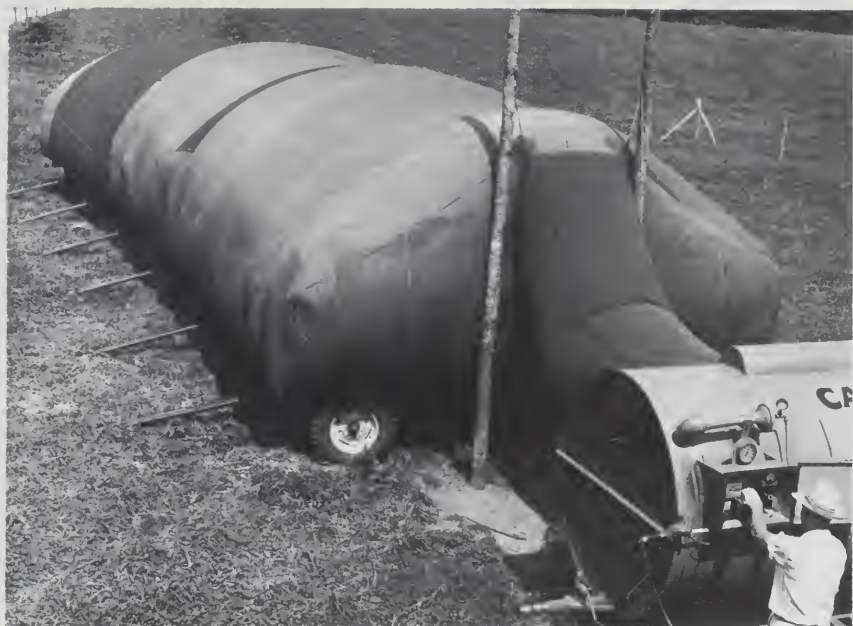
A hay drier developed at the North Carolina Agricultural Experiment Station.
